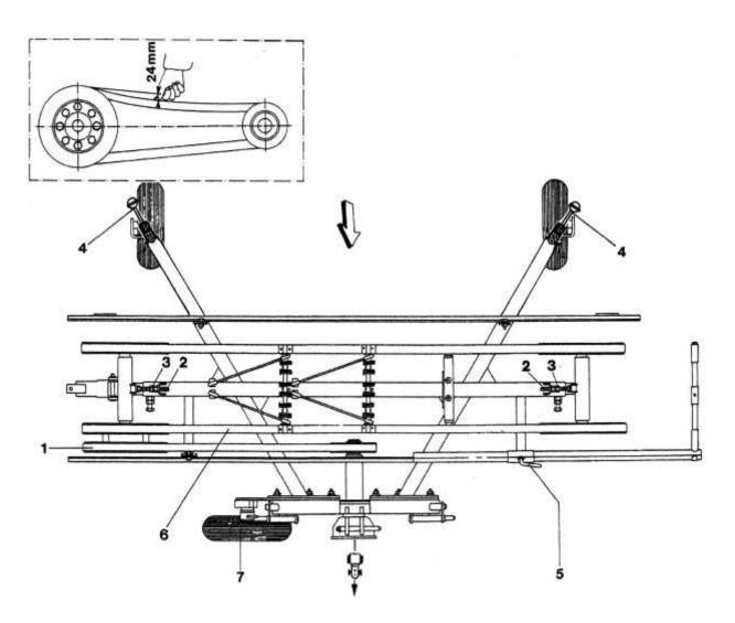
Figure 2 Belt hay rake - tightening belts
