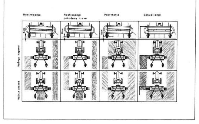
Figure 5. working height regulation
